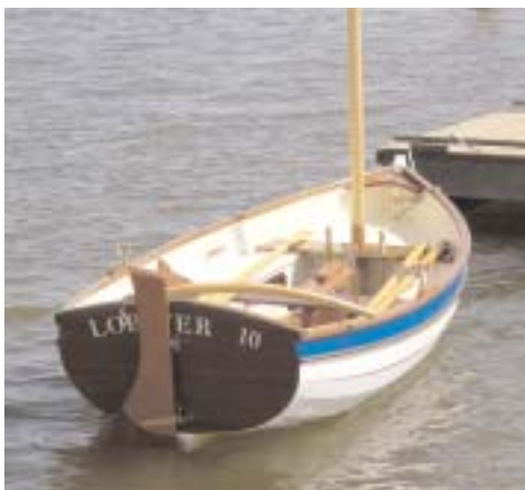
Bart's second design in his Lobster range is this 10' (3m) transom-stern clinker dinghy.
